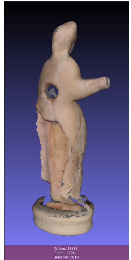
Fig. 3. Processing 3-D scans: The scan after noise removal
